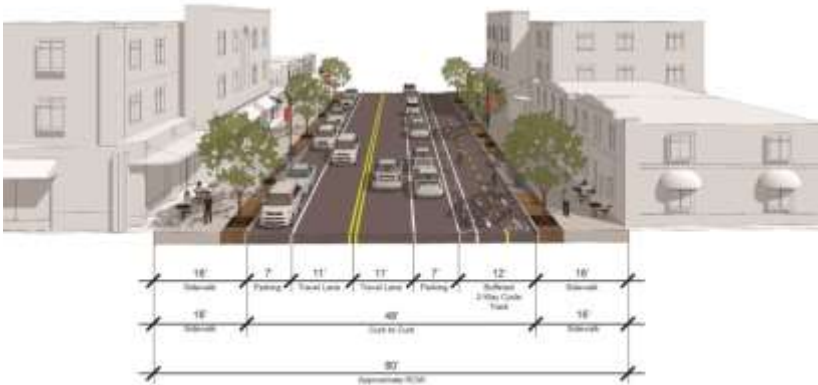
Penn Street: Proposed Typical Cross-Section Option2: Two-Way Cycle Track
