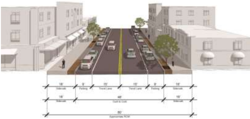
Penn Street: Existing Typical Cross-Section
