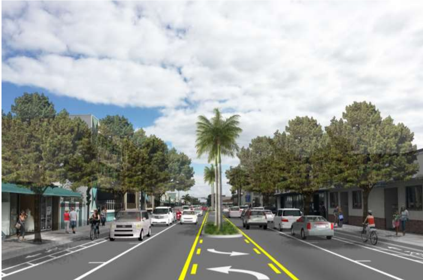
Option 1: Three Lanes with Spot Medians, Parking, and Buffered Bike lanes
