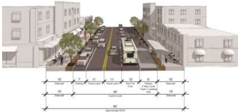
Penn Street: Proposed Typical Cross-Section Option2: Two-Way Cycle Track and Eastbound Bus Stop
