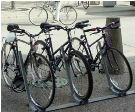
Wheel well secured racks. Not recommended. (Photos: Arthur Ross, City of Madison; Creative Pipe, Inc.; John Cinatl)
