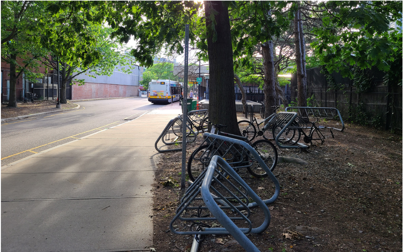
ADA-compliant access routes and clear space around racks are essential for making bike parking usable for diverse riders (Photo: Alyson Fletcher)
